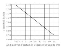
To use this chart: Read up from the ambient temperature to the curve, and across to find a correction factor. Multiply the breaker rating by the correction factor to determine the compensated rating. Calculate the overloads in terms of the compensated
