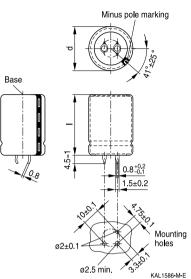
Snap-in terminals, length  $(6.3 \pm 1)$  mm. Also available in a shorter version with a length of (4.5 - 1) mm. PET insulation is marked with label "PET" on the sleeve. Safety vent on the case wall.
