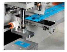
Bergquist Sil-Pad 1500ST (Soft Tack) is a fiberglass reinforced thermal interface material that is naturally tacky on both sides. Sil-Pad 1500ST exhibits superior thermal performance when compared to the competitors' thermal interface materials. Sil-Pad 1500ST is supplied in sheet or roll form for exceptional auto-dispensing and auto-placement in high volume assemblies. Sil-Pad 1500ST is intended for placement between an electronic power device and its heat sink.
